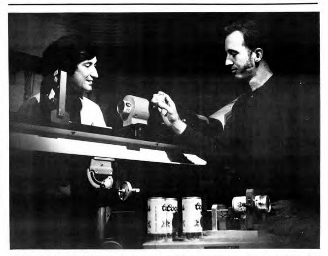
COLLAPSED ALUMINUM BEER CAN is examined by Art Van Hook (8156), right, and Gene Neau (8416) after the can was used in the fast shutter system they developed to eliminate rewrite problems inherent in high speed cameras.
